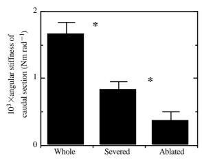
Fig. 6. Stiffness of the body is altered by changes in locomotor morphology. Profile analysis of variance (N=3) was used to analyze the data from the mechanical bending tests, with three experimental treatment categories in the independent variable and angular stiffness as the dependent variable. The two comparisons revealed a significant drop in stiffness with each treatment category. The asterisks indicate a significant difference between the means at P<0.05. Bars show S.E.M.
