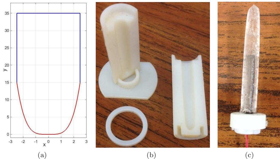
Figure 2. Fabrication of cupula-like structure: (a) shape design; (b) 3D-printed mold parts; (c) IPMC sensor coated with cupula-like PDMS.
