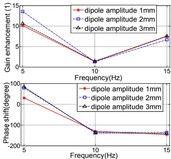
Figure 4. Experimental results for the improvement of sensor performance under periodic flow stimulus.
