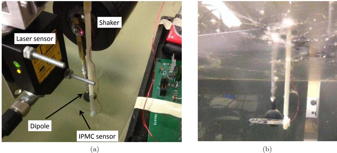
Figure 3. Experimental setup with a dipole source: (a) top view; (b) side view.
